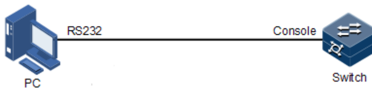
Figure 1-1 Accessing device through PC connected with RJ45 Console interface
