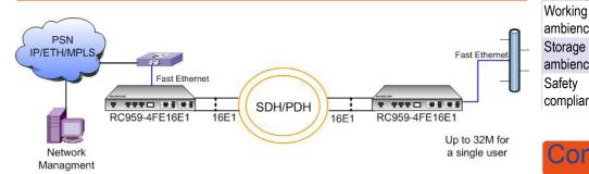
Scenario 1 presents a typical solution for transmitting one Fast Ethernet over 16 bonded E1 circuits, increasing the bandwidth of a single subscriber up to 32M. By adopting international GFP protocol for encapsulation, RC959-4FE16E1 satisfies the demand of enterprise customer conveniently by utilizing existing TDM network resource cost-efficiently.
