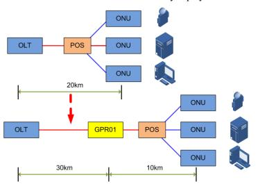
2. It is deployed between the OLT and optical splitter to increase optical splitting ratio, which can resolve the optical splitting ratio limit problem due to inadequate optical budget.
